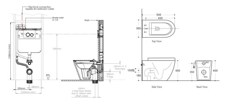
Note: Toilet pan dimensions may vary slightly due to tolerances in the manufacturing process. Please check exact dimensions on actual pan.
