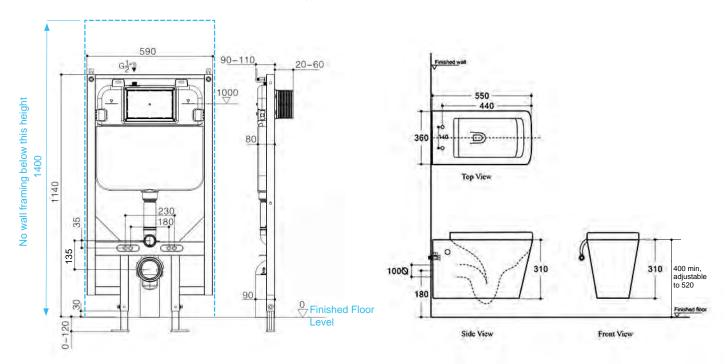
Note: Toilet pan dimensions may vary slightly due to tolerances in the manufacturing process. Please check exact dimensions on actual pan,
